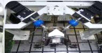
Right & Left Back 45 deg Moment Durability Test
