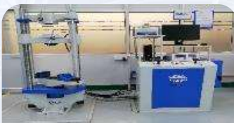
Tensile, Elongation, Yield, Compression Test and Bend
