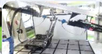
Forward & Backward Moment Durability Test
