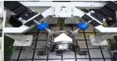
Right & Left Back 45 deg Moment Durability Test
