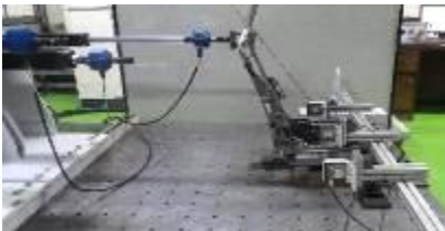
Horizontal Backward Moment Loading Test (Strength Test)
