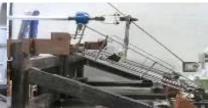
Armrest Downward Strength Test
